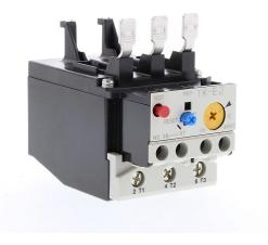
Fuji Electric TK-E2 series thermal overload relay, 7.0-11.0A adjustable, bi-metallic, direct mount power connection(s). For use with SC-E1x, SC-E2x and SC-E2Sx contactors.
