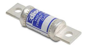
Edison fuse, TJS series, Class T, current-limiting, extremely fastacting, 90A, 600 VAC, knife blade. Package of 5. Feeder/branch, semiconductor protection applications.
