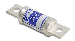
Edison fuse, TJS series, Class T, current-limiting, extremely fast-acting, 80A, 600 VAC, knife blade. Package of 5. Feeder/branch, semiconductor protection applications.
