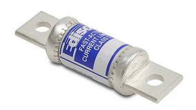
Edison fuse, TJS series, Class T, current-limiting, extremely fast-acting, 80A, 600 VAC, knife blade, feeder/branch, semiconductor protection applications.
