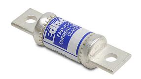
Edison fuse, TJS series, Class T, current-limiting, extremely fast-acting, 80A, 600 VAC, knife blade, feeder/branch, semiconductor protection applications.
