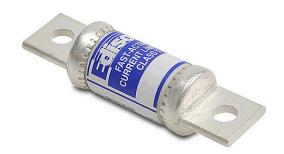
Edison fuse, TJS series, Class T, current-limiting, extremely fast-acting, 70A, 600 VAC, knife blade. Package of 5. Feeder/branch, semiconductor protection applications.
