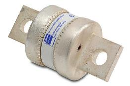
Edison fuse, TJS series, Class T, current-limiting, extremely fastacting, 500A, 600 VAC, knife blade, feeder/branch, semiconductor protection applications.
