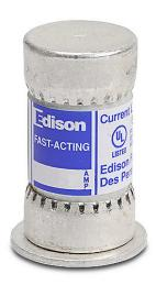
Edison fuse, TJS series, Class T, current-limiting, extremely fast-acting, 50A, 600 VAC, ferrule, feeder/branch, semiconductor protection applications.
