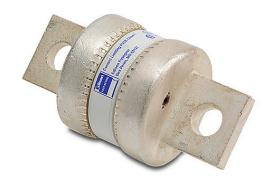
Edison fuse, TJS series, Class T, current-limiting, extremely fast-acting, 450A, 600 VAC, knife blade, feeder/branch, semiconductor protection applications.
