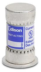
Edison fuse, TJS series, Class T, current-limiting, extremely fastacting, 45A, 600 VAC, ferrule, feeder/branch, semiconductor protection applications.
