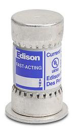
Edison fuse, TJS series, Class T, current-limiting, extremely fast-acting, 40A, 600 VAC, ferrule. Package of 10. Feeder/branch, semiconductor protection applications.
