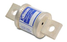
Edison fuse, TJS series, Class T, current-limiting, extremely fast-acting, 400A, 600 VAC, knife blade, feeder/branch, semiconductor protection applications.
