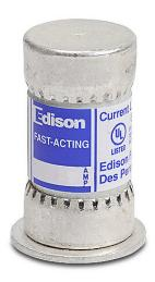
Edison fuse, TJS series, Class T, current-limiting, extremely fast-acting, 40A, 600 VAC, ferrule, feeder/branch, semiconductor protection applications.
