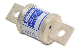
Edison fuse, TJS series, Class T, current-limiting, extremely fastacting, 350A, 600 VAC, knife blade, feeder/branch, semiconductor protection applications.
