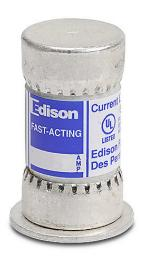
Edison fuse, TJS series, Class T, current-limiting, extremely fast-acting, 35A, 600 VAC, ferrule, feeder/branch, semiconductor protection applications.
