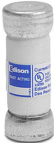
Edison fuse, TJS series, Class T, current-limiting, extremely fast-acting, 25A, 600 VAC, ferrule. Package of 10. Feeder/branch, semiconductor protection applications.
