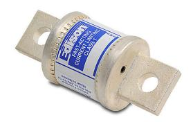
Edison fuse, TJS series, Class T, current-limiting, extremely fast-acting, 250A, 600 VAC, knife blade, feeder/branch, semiconductor protection applications.
