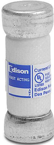
Edison fuse, TJS series, Class T, current-limiting, extremely fast-acting, 20A, 600 VAC, ferrule, feeder/branch, semiconductor protection applications.
