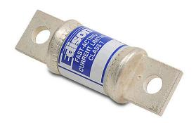
Edison fuse, TJS series, Class T, current-limiting, extremely fast-acting, 110A, 600 VAC, knife blade, feeder/branch, semiconductor protection applications.
