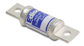
Edison fuse, TJS series, Class T, current-limiting, extremely fastacting, 100A, 600 VAC, knife blade. Package of 5. Feeder/branch, semiconductor protection applications.
