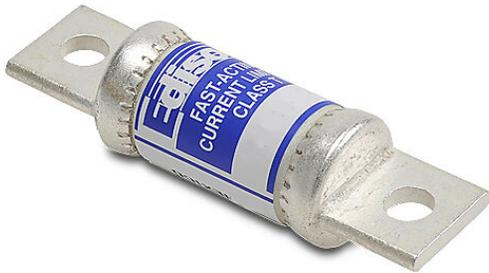
Edison fuse, TJS series, Class T, current-limiting, extremely fast-acting, 100A, 600 VAC, knife blade, feeder/branch, semiconductor protection applications.
