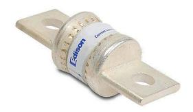
Edison fuse, TJN series, Class T, current-limiting, extremely fast-acting, 90A, 300 VAC, knife blade. Package of 5. Feeder/branch, semiconductor protection applications.
