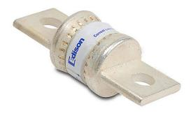
Edison fuse, TJN series, Class T, current-limiting, extremely fastacting, 90A, 300 VAC, knife blade. Package of 5. Feeder/branch, semiconductor protection applications.
