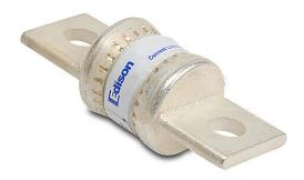
Edison fuse, TJN series, Class T, current-limiting, extremely fastacting, 90A, 300 VAC, knife blade, feeder/branch, semiconductor protection applications.
