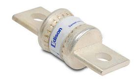
Edison fuse, TJN series, Class T, current-limiting, extremely fast-acting, 80A, 300 VAC, knife blade. Package of 5. Feeder/branch, semiconductor protection applications.
