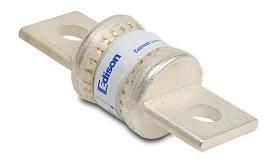
Edison fuse, TJN series, Class T, current-limiting, extremely fastacting, 80A, 300 VAC, knife blade, feeder/branch, semiconductor protection applications.
