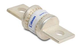
Edison fuse, TJN series, Class T, current-limiting, extremely fast-acting, 70A, 300 VAC, knife blade, feeder/branch, semiconductor protection applications.
