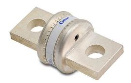
Edison fuse, TJN series, Class T, current-limiting, extremely fast-acting, 600A, 300 VAC, knife blade, feeder/branch, semiconductor protection applications.
