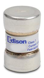
Edison fuse, TJN series, Class T, current-limiting, extremely fast-acting, 60A, 300 VAC, ferrule, feeder/branch, semiconductor protection applications.
