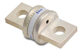
Edison fuse, TJN series, Class T, current-limiting, extremely fastacting, 500A, 300 VAC, knife blade, feeder/branch, semiconductor protection applications.
