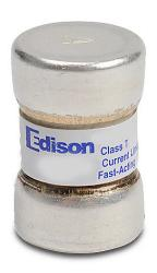
Edison fuse, TJN series, Class T, current-limiting, extremely fast-acting, 50A, 300 VAC, ferrule, feeder/branch, semiconductor protection applications.
