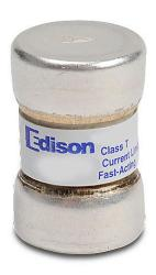
Edison fuse, TJN series, Class T, current-limiting, extremely fast-acting, 45A, 300 VAC, ferrule. Package of 10. Feeder/branch, semiconductor protection applications.
