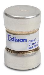
Edison fuse, TJN series, Class T, current-limiting, extremely fast-acting, 45A, 300 VAC, ferrule, feeder/branch, semiconductor protection applications.
