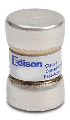
Edison fuse, TJN series, Class T, current-limiting, extremely fast-acting, 40A, 300 VAC, ferrule. Package of 10. Feeder/branch, semiconductor protection applications.
