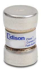
Edison fuse, TJN series, Class T, current-limiting, extremely fast-acting, 35A, 300 VAC, ferrule, feeder/branch, semiconductor protection applications.
