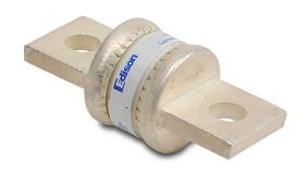
Edison fuse, TJN series, Class T, current-limiting, extremely fast-acting, 200A, 300 VAC, knife blade, feeder/branch, semiconductor protection applications.
