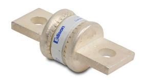
Edison fuse, TJN series, Class T, current-limiting, extremely fast-acting, 150A, 300 VAC, knife blade, feeder/branch, semiconductor protection applications.
