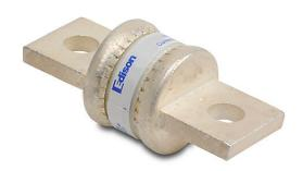
Edison fuse, TJN series, Class T, current-limiting, extremely fast-acting, 110A, 300 VAC, knife blade, feeder/branch, semiconductor protection applications.
