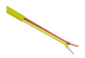
TE Wire & Cable Type K thermocouple PLTC extension wire, unshielded, 2 conductors, 20 AWG, nickel-chromium and nickel-aluminum, PVC conductor insulation material, yellow and red, PVC jacket, yellow, cut to length.
