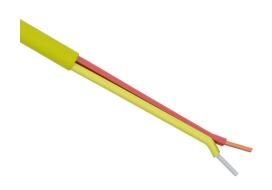
TE Wire & Cable Type K thermocouple PLTC extension wire, unshielded, 2 conductors, 20 AWG, nickel-chromium and nickel-aluminum, PVC conductor insulation material, yellow and red, PVC jacket, yellow, cut to length.
