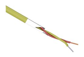
TE Wire & Cable Type K thermocouple PLTC extension wire, shielded, 2 conductors, 16 AWG, nickel-chromium and nickel-aluminum, FEP Teflon conductor insulation material, yellow and red, FEP Teflon jacket, yellow, cut to length.
