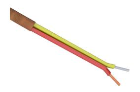
TE Wire & Cable Type K thermocouple extension wire, unshielded, 2 conductors, 20 AWG, nickel-chromium and nickel-aluminum, high temperature fiberglass conductor insulation material, yellow and red, high temperature fiberglass jacket, brown, cut to length.
