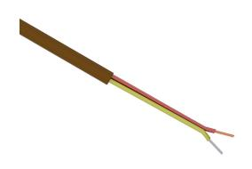
TE Wire & Cable Type K thermocouple extension wire, unshielded, 2 conductors, 20 AWG, nickel-chromium and nickel-aluminum, FEP Teflon conductor insulation material, yellow and red, FEP Teflon jacket, brown, cut to length.
