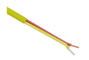
TE Wire & Cable Type K thermocouple extension wire, unshielded, 2 conductors, 16 AWG, nickel-chromium and nickel-aluminum, PVC conductor insulation material, yellow and red, PVC jacket, yellow, cut to length.
