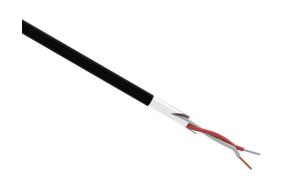
TE Wire & Cable Type J thermocouple PLTC extension wire, shielded, 2 conductors, 20 AWG, iron and copper-nickel, FEP Teflon conductor insulation material, white and red, FEP Teflon jacket, black, cut to length.
