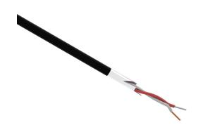
TE Wire & Cable Type J thermocouple PLTC extension wire, shielded, 2 conductors, 16 AWG, iron and copper-nickel, PVC conductor insulation material, white and red, PVC jacket, black, cut to length.
