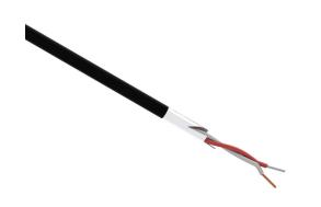
TE Wire & Cable Type J thermocouple PLTC extension wire, shielded, 2 conductors, 16 AWG, iron and copper-nickel, FEP Teflon conductor insulation material, white and red, FEP Teflon jacket, black, cut to length.
