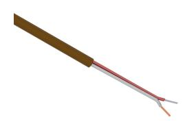
TE Wire & Cable Type J thermocouple extension wire, unshielded, 2 conductors, 20 AWG, iron and copper-nickel, FEP Teflon conductor insulation material, white and red, FEP Teflon jacket, brown, cut to length.
