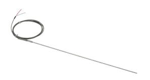
ProSense temperature sensor, Type T thermocouple, lead wire transition probe, ungrounded, 18in insertion length, 1/8in probe diameter, stainless steel sheath, 6ft 20 AWG wire leads.
