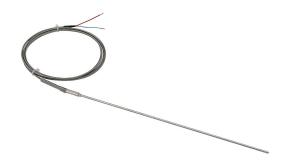
ProSense temperature sensor, Type T thermocouple, lead wire transition probe, ungrounded, 12in insertion length, 1/8in probe diameter, stainless steel sheath, 6ft 20 AWG wire leads.
