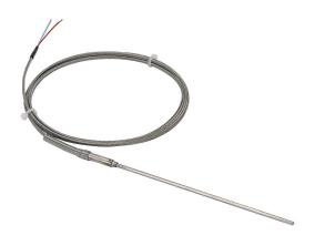
ProSense temperature sensor, Type T thermocouple, lead wire transition probe, ungrounded, 6in insertion length, 1/8in probe diameter, stainless steel sheath, 6ft 20 AWG wire leads.
