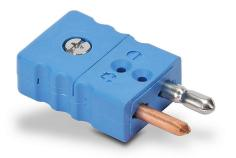
ProSense Type T thermocouple connector, standard round pin plug, 400 deg F (200 deg C), glass filled thermoplastic body, blue, thermocouple material pins, 32 AWG to 14 AWG wire size range.
