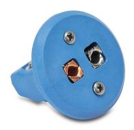
ProSense Type T thermocouple connector, standard round pin panel jack, 400 deg F (200 deg C), glass filled thermoplastic body, blue, thermocouple material pins, 32 AWG to 14 AWG wire size range.
